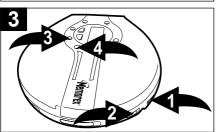
Adjust the VOLUME control ● and DBBS switch ❷ as desired. To **skip** forward or backward through the tracks on the disc, press the SKIP/SEARCH |◀◀ ❸ or ▶▶ button ④. To **search** forward or backward through the tracks on the disc, press and hold the SKIP/SEARCH |◀◀ ❸ or ▶▶ button ④.
